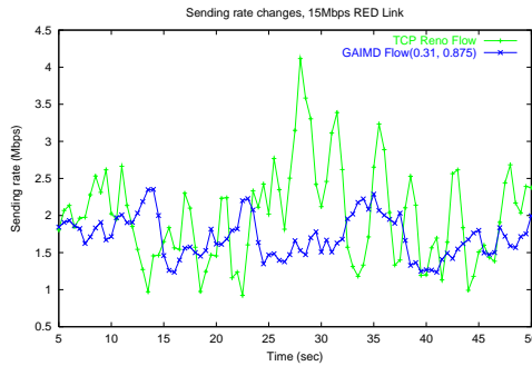
Figure 21: GAIMD and TCP sending rate traces for a 15Mbps RED link
