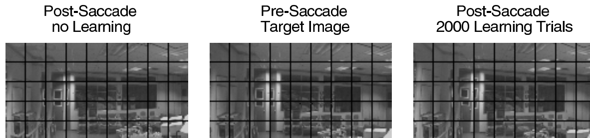
Figure 6: Expanded example of the visual learning of the saccade map. The center collage is the pre-saccade target images \bar{I}_t for a subset of the entire saccade map. The left collage shows the post-saccade image centers with no learning. The right collage shows the post-saccade image centers after 2000 learning trials. The post-learning collage shows a much better match to the target than the pre-learning collage.
