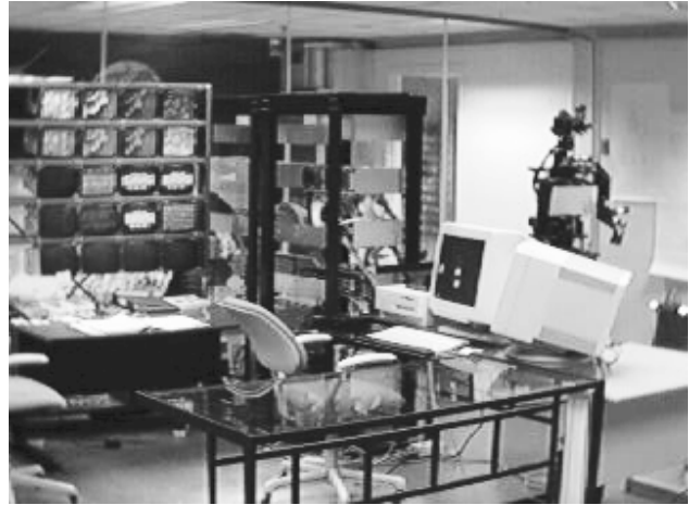
Figure 2: Supporting structure for Cog. The "brain" of the robot is a MIMD computer which occupies the racks in the center of this image. Video from the cameras or from the brain is displayed on a bank of twenty displays shown on the left. User interface and file storage are provided by a Macintosh Quadra. Cog itself is on the far right.
