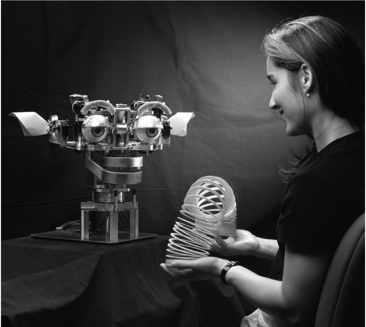
Figure 1. Kismet with toys. Kismet has an active stereo vision system with color CCD cameras mounted inside the eyeballs. There are also a variety of facial features which give the robot its expressive capabilities.
