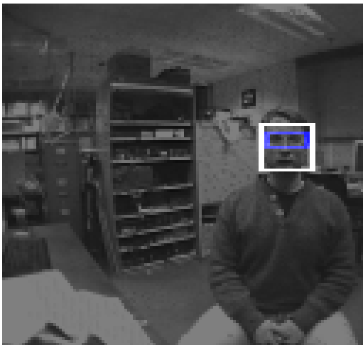
Figure 6. An example face in a cluttered environment. The 128×128 grayscale image was captured by the active vision system and then processed by the pre-filtering and ratio template detection routines. One face was found within the image, and is shown outlined.
