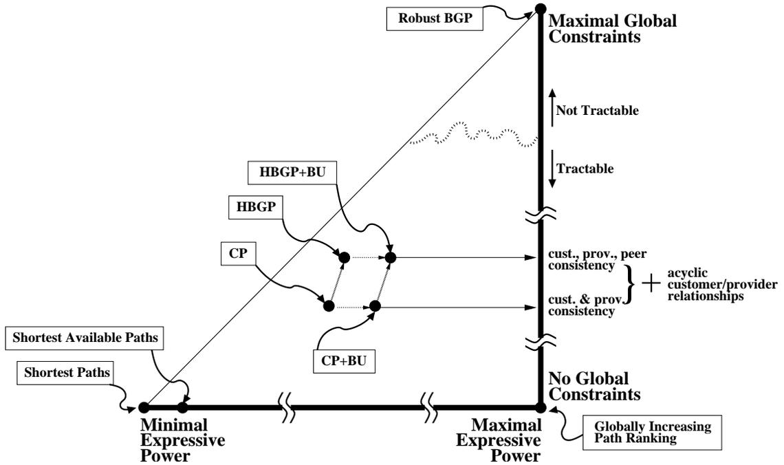
Figure 4.1: Design space for robust path-vector systems.
