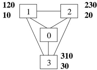
Figure 3.1: The routing configuration (SPP instance) BAD GADGET.
