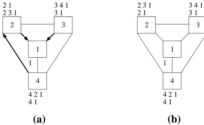
Figure 4.5: (a) The SPP GOOD GADGET and its unique solution shown in bold. (b) The SPP BAD GADGET.
