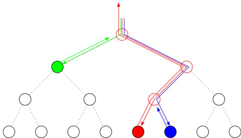
**Adaptive test-and-set** on a binary tree of depth  $3 \log_2 n$ .
